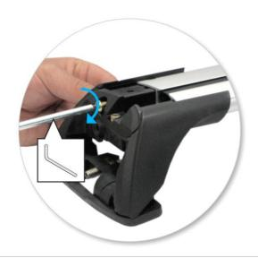
• Tighten adjusting screw to 5 Nm.
